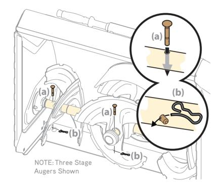
Shear pins are designed to break if the snow blower hits a hard object preventing damage to more expensive parts.
